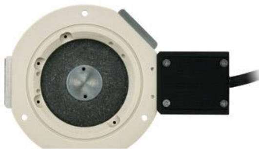
Figure 5.8 MFP-3D PolyHeater stage, the stage consists of a metal heating element 1.5cm in diameter (centre of the image) surrounded by a Teflon insulating layer (inner black ring) which is then framed by a Polyether ether ketone (PEEK) support (beige outer ring). This heating stage is designed to allow in-situ AFM measurements at elevated temperature in air or a controlled gas environment. Allows heating from room temperature to 300^{\circ}\text{C} . [38]
