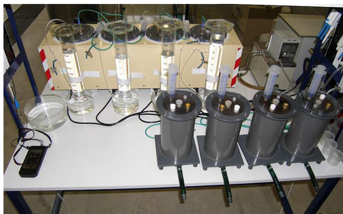
Figure 1: Photo of pilot plan with 8 aerobic and anaerobic reactors.
