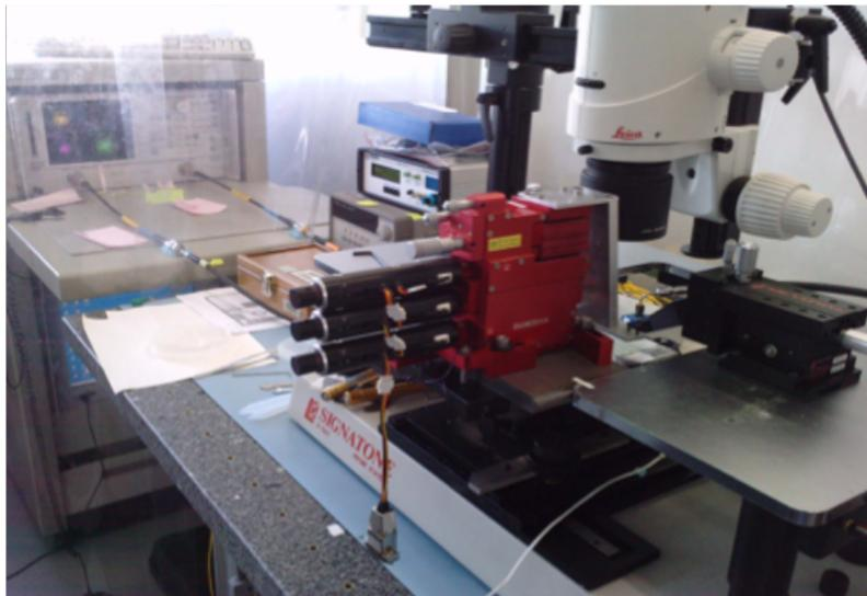
Figure 2.27 On- wafer DC and RF characterization bench
