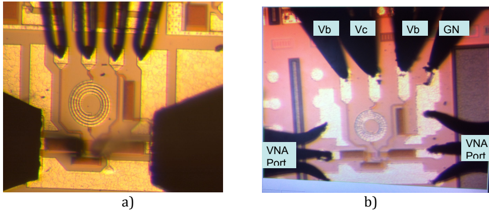
Figure 5.17 HPT in cascode in a) 150µm pitch GSG Pads b) 200µm pitch pads
