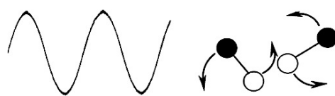
Fig. 43. Dipolar molecules that try to align with an oscillating electromagnetic field. 240
