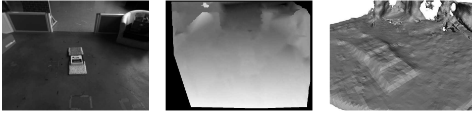
Figure 4.31 – From a pair of images of the scene in front of the robot (left) a dense disparity map is estimated (middle) and from this disparity map a dense surface integrating the previous frames into the volumetric grid is estimated (right). These images were taken from the HRP-2 stereo vision system with the cameras tilted towards the ground to allow ground reconstruction tasks. It is assumed that a mechanism is implemented to make the robot search for traversable areas [Maier 13].
