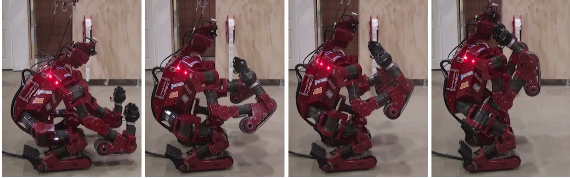
Figure 4.46 – CHIMP moving to its final 2 limb posture (second part of posture change from four limbs to two limbs)
