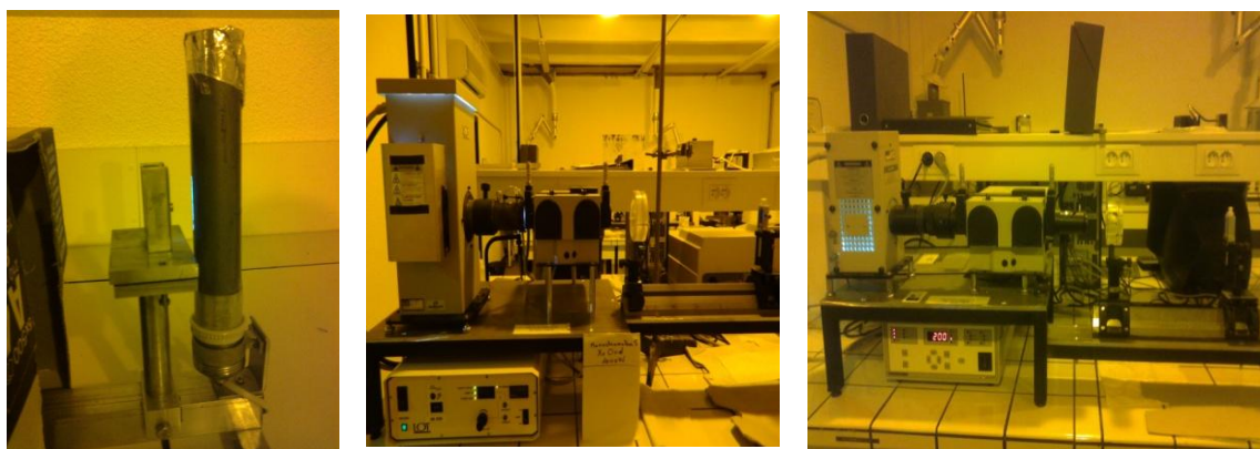
Figure 8-1 Irradiation monochromatic systems: 254 nm (left), 300 and 310 nm (centre) and at 313 and 365 nm (right).
