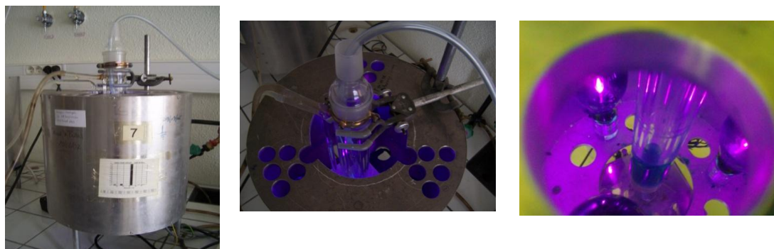
Figure 8-3 Irradiation system at 365 nm with 3 wood lamps.
