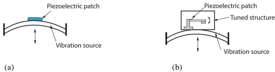
Figure 3-1. The direct energy harvesting (a) and indirect energy harvesting (b)
