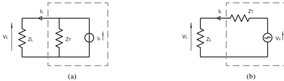
Figure 2-5. Piezoelectric harvester equivalent circuit (Piezoelectric generator with load) using Norton (a) or Thevenin (b) representations
