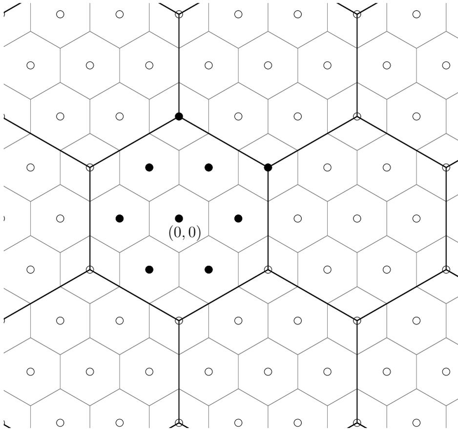
Figure 4.1: A Voronoi constellation of the hexagonal lattice in dimension 2. Filled and empty circles are the points of  $\Lambda_f$ . Small hexagons represent their Voronoi regions. Big hexagons are the Voronoi regions of  $\Lambda = 3\Lambda_f$ . The filled circles are the  $3^2 = 9$  points of the constellation  $\Lambda_f/\Lambda$ , contained in  $\mathcal{V}(\Lambda)$ .
