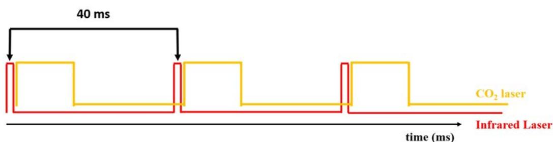
Figure 1-12: Synchronization of the tunable infrared lasers (red) with the auxiliary cw CO<sub>2</sub> laser (yellow). A few  $\mu$ s after irradiation by the infrared tunable laser, ions are irradiated with a pulse of the cw CO<sub>2</sub> laser. The CO<sub>2</sub> laser pulse is typically few milliseconds long.
