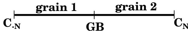
Figure 3.7: Bicrystal type membrane considered in the simulation of 1D diffusion across the grain boundary.
