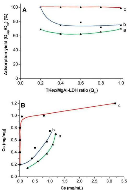
**Fig. 1.** (A) Adsorption yield ( $Q_{ex}/Q_{th}$ ) as a function of TKec:LDH ratio ( $Q_{th}$ ) and (B) adsorption isotherms of TKec on Mg<sub>2</sub>Al-NO<sub>3</sub> in H<sub>2</sub>O (a), 50 mM MOPS (b), and 100 mM Gly-Gly (c).
