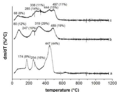
Fig. 5. Differential thermal gravimetry analysis (DTG) of (a) MgAl-Gly-Gly<sub>cop</sub>, (b) TKec@MgAl-Gly-Gly<sub>cop</sub> (Mg:Al = 2), (c) TKec@MgAl-Gly-Gly<sub>ads</sub> pH 7.5.
