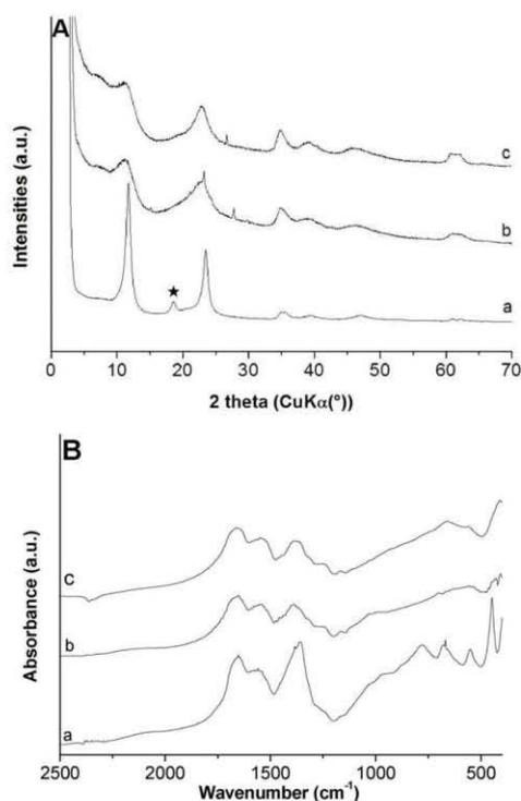
Fig. 4. (A) X-ray diffraction patterns of TKec@MgAl-Gly-Gly<sub>ads</sub> pH 7.5 (a), TKec@Mg<sub>2</sub>Al-Gly-Gly<sub>cop</sub> (b) and TKec@Mg<sub>4</sub>Al-Gly-Gly<sub>cop</sub> (c). (B) FTIR spectra of TKec@MgAl-Gly-Gly<sub>ads</sub> pH 7.5 (a), TKec@MgAl-Gly-Gly<sub>cop</sub> (Mg:Al = 2) (b) and TKec@MgAl-Gly-Gly<sub>cop</sub> (Mg:Al = 4) (c).
