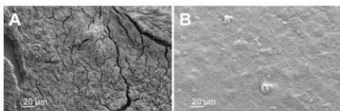
**Fig. 7.** SEM images of films of TKec@MgAl-Gly-Gly<sub>cop</sub> prepared in 100 (a) and 25 (b) mM Gly-Gly.
