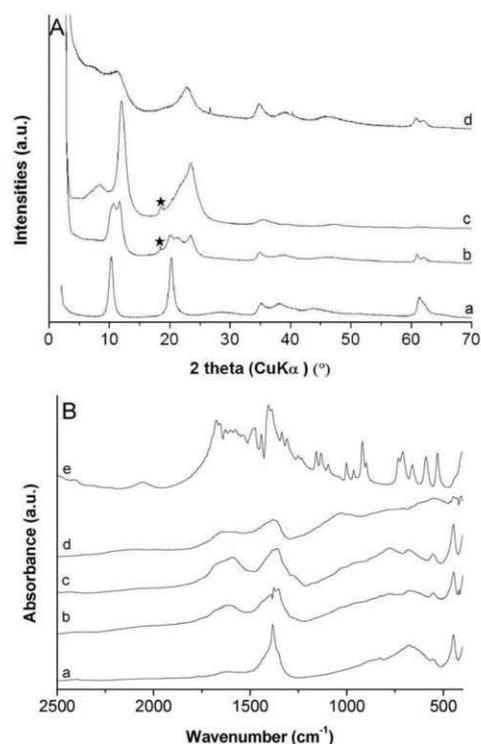
Fig. 3. (A) X-ray diffraction patterns of Mg<sub>2</sub>Al-NO<sub>3</sub> (a), MgAl-Gly-Gly pH 7.5 (b), MgAl-Gly-Gly pH 9.0 (c) and MgAl-Gly-Gly<sub>cop</sub> (d), (\* by-product). (B) FTIR spectra of Mg<sub>2</sub>Al-NO<sub>3</sub> (a), MgAl-Gly-Gly pH 7.5 (b), MgAl-Gly-Gly pH 9.0 (c), MgAl-Gly-Gly<sub>cop</sub> (d), and Gly-Gly (e).
