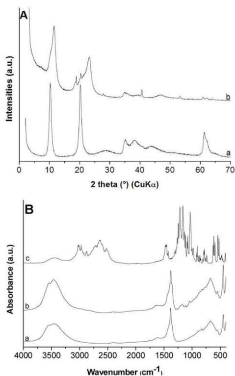
Fig. 2. (A) X-ray diffraction patterns of Mg<sub>2</sub>Al-NO<sub>3</sub> (a) and MgAl-MOPS (b). (B) FTIR spectra of Mg<sub>2</sub>Al-NO<sub>3</sub> (a), MgAl-MOPS (b) and MOPS (c).
