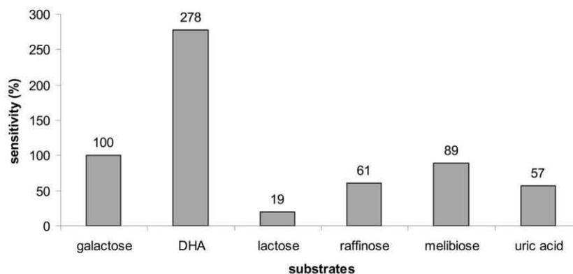
Fig. 2. Relative response of the GAOx/laponite (25:50;  $\mu\text{g}:\mu\text{g}$ ) biosensors for different substrates. Mean response of 5 injections of substrate at 20  $\mu\text{M}$ . Other experimental conditions: HEPES pH 7.0; 50 mM, 25°.
