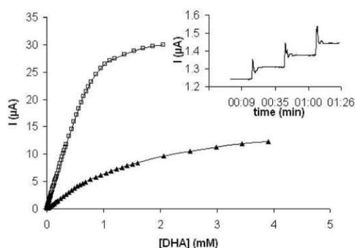
Fig. 1. Calibration curves for dihydroxyacetone (DHA) recorded at the a) GAOx/laponite electrode ( $\square$ ) and b) GAOx/ $\text{MgAl-NO}_3$  (50:50;  $\mu\text{g}:\mu\text{g}$ ) electrodes ( $\blacktriangle$ ). Other experimental conditions: HEPES pH 7.0; 50 mM, 25 °C. Inset: Steady-state anodic current-time responses of GAOx/laponite (50:50;  $\mu\text{g}:\mu\text{g}$ ) electrode for 2  $\mu\text{M}$  DHA additions.
