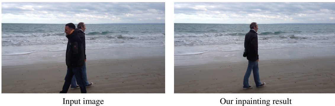
FIGURE 2.2: An example of results of video inpainting (using the algorithm proposed in Chapter 6). The person in the foreground has been removed from the video.
