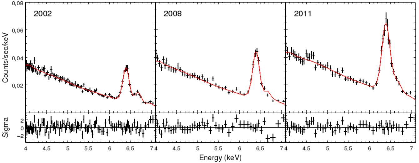
**Fig. 3.** Bridge spectra and fit as in 2002 (no bright illumination seen in the Bridge), 2008 (illumination starts in the western part of Br1) and 2011 (illumination reaches Br2). The Fe  $K\alpha$  flux is significantly increasing over the years.
