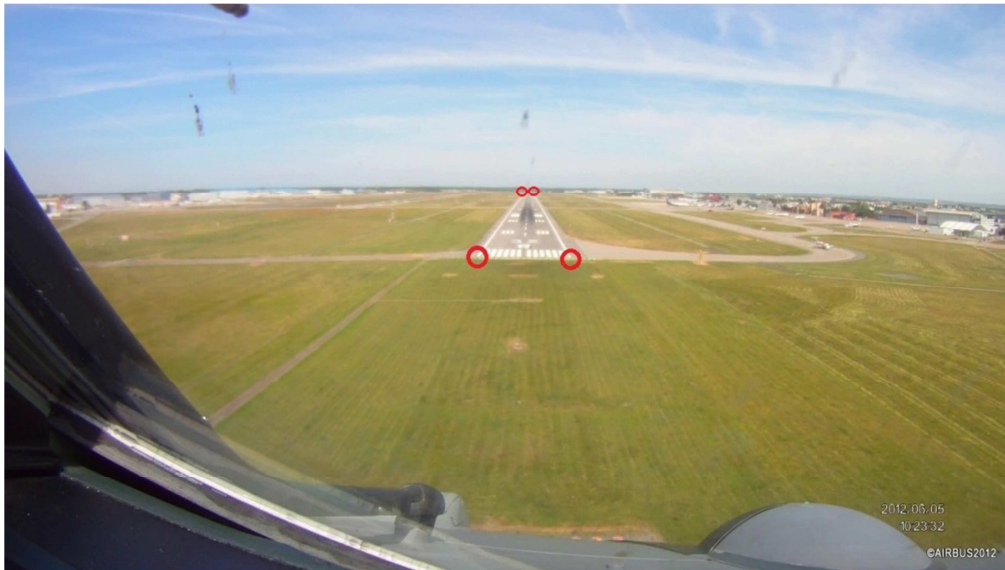
Figure 29 – Runway's corners detection during landing taken at 230m of the runway's threshold
