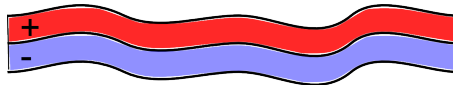
FIGURE 2.4: Schematic section of a bimorph mirror: the positive polarization is represented in red and the negative polarization is in blue. The laser beam can be reflected on one side or the other depending on the coating position.
