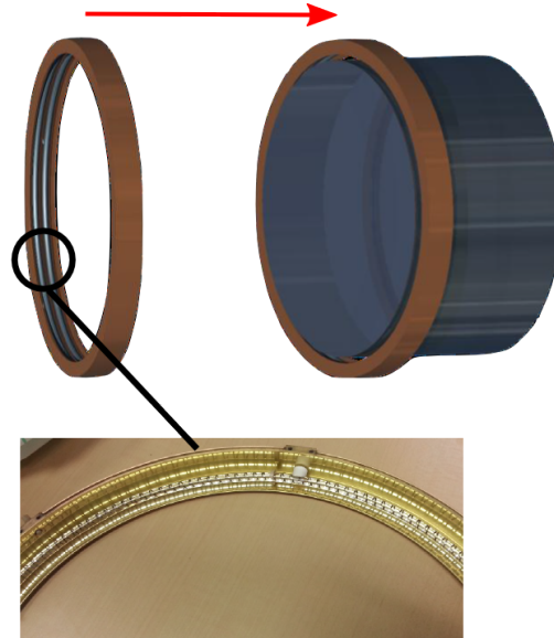
FIGURE 2.8: Scheme of the ring heater position around a test mass. The ring heater is composed of two emitting elements inside a circular shield. In the zoom picture, the annular element of the prototype is made of glass and is surrounded by a gold coated copper shield. Pictures are from the Advanced Virgo TCS group
