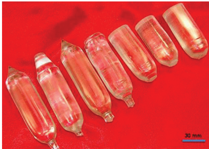
Figure 3.2 The as grown sapphire crystals grown by Cz method
