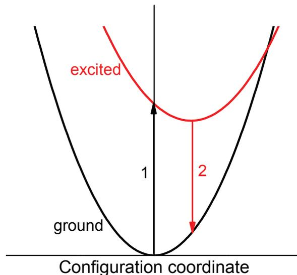
Figure 1.13: *Configuration diagram of a luminescent center*
