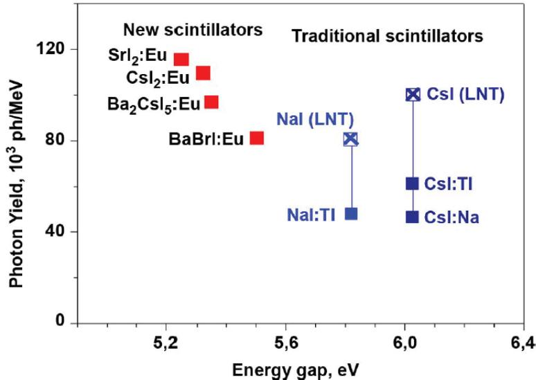
Figure I1: *Estimation of scintillation efficiency of halide scintillators*
