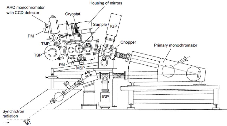
Figure 2.7: *Side view of the SUPERLUMI setup*
