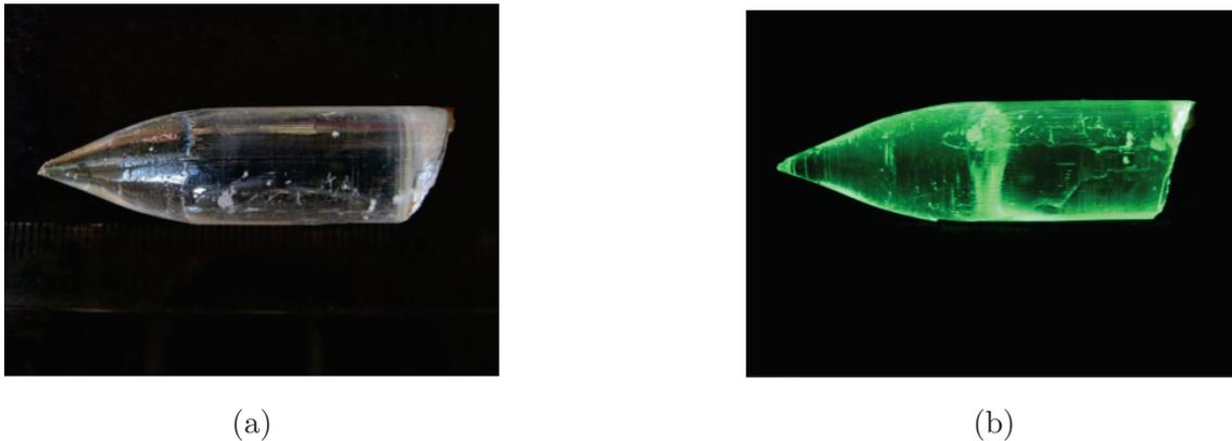
Figure 2.2: *CsI:In* single crystal under day light (a) and under UV light (b)
