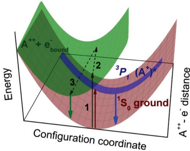
Figure 3.12: *Configuration diagram of activator relaxation in CsI:A with account of the spatial coordinate*
