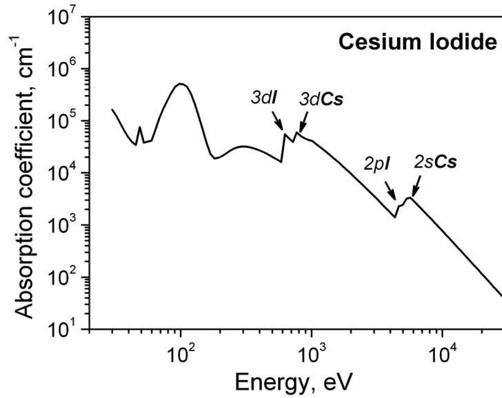
Figure 1.4: *Electromagnetic energy absorption coefficient in the X-ray energy range for CsI [xRa, 2014]*
