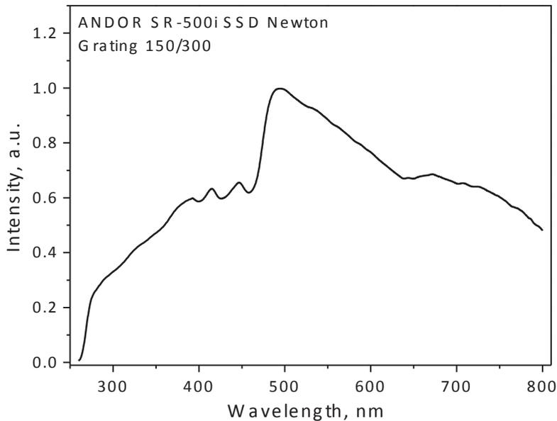
Figure 2.8: *Spectral sensitivity of the ANDOR Newton CCD coupled with Shamrock 500i spectrograph*
