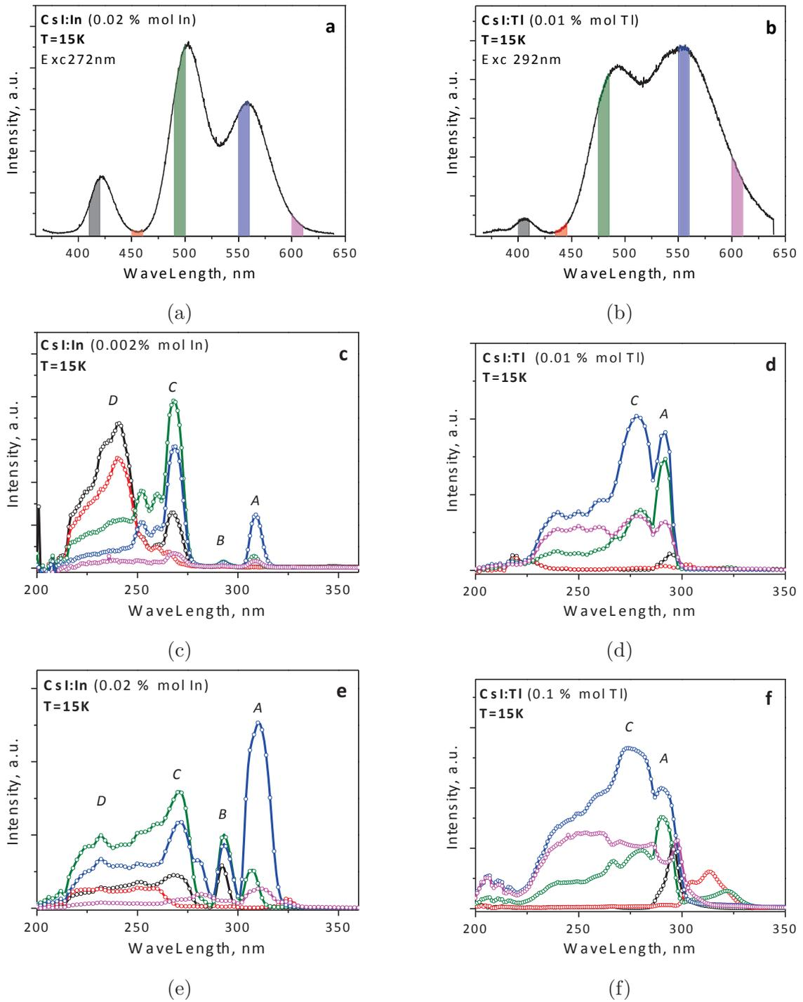
Figure 3.4: Activator luminescence spectra of CsI:In under 272nm excitation (a), and CsI:Tl under 292nm excitation (b) measured at 15 K. Excitation spectra of CsI:In activator luminescence (c, e) and CsI:Tl crystal (d, f) for the respective segments of the emission bands
