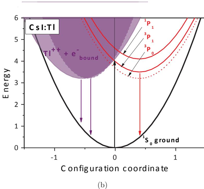
Figure 3.9: Configuration diagrams for CsI:In (a) and CsI:Tl (b)
