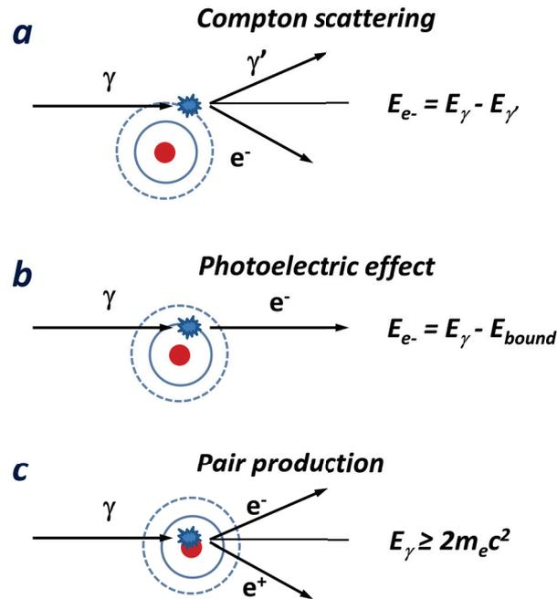
Figure 1.2: *Three different types of interaction of ionizing radiation with matter [Evans, 1955]. a – Compton effect, b – photoelectric effect, c – pair production*
