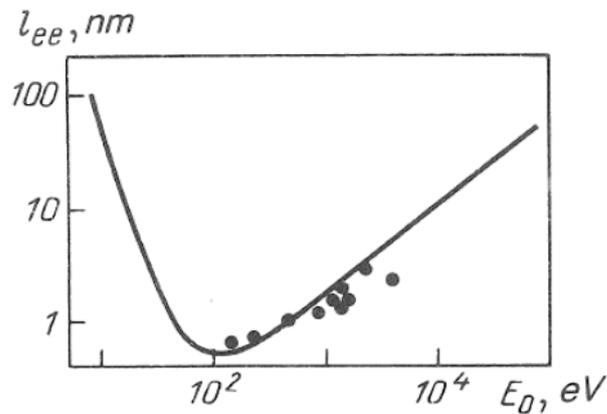
Figure 1.5: *Mean free path of electrons in the case of inelastic scattering by bound electrons in  $Al_2O_3$  (the points are the experimental results) [Ritchie et al., 1975]*
