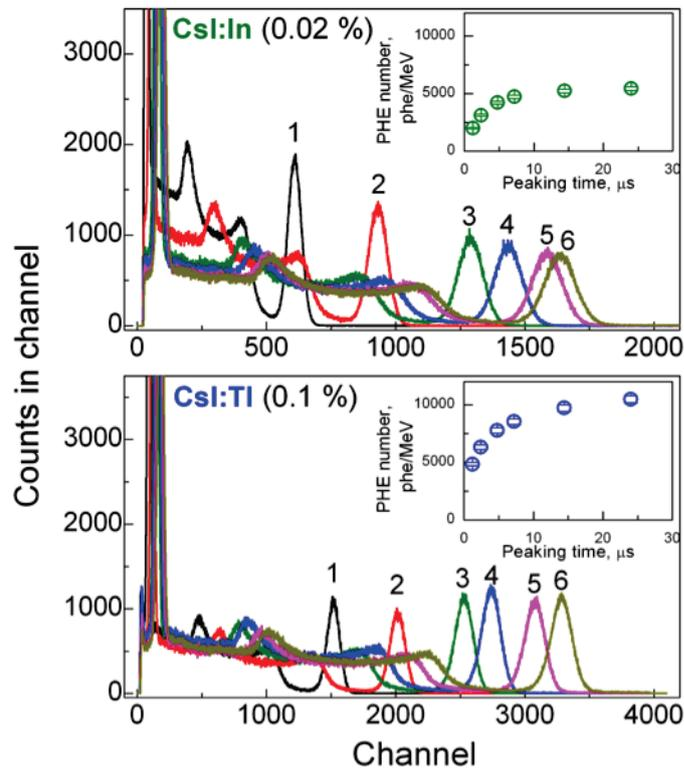
Figure 4.1: Pulse height spectra of CsI:In (a) and standard CsI:Tl (b) measured with different peaking times under  $^{137}\text{Cs}$   $\gamma$ -excitation of 661.6 keV. Insets - photoelectron number as a function of the integration gate
