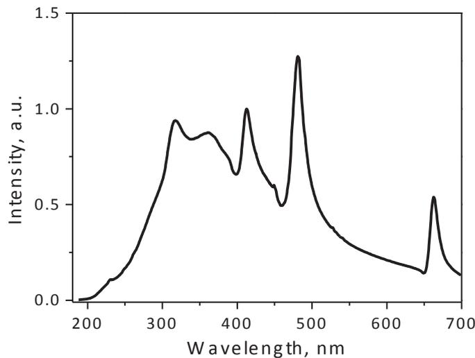
Figure 2.6: *The spectrum of the UV excitation optical system*
