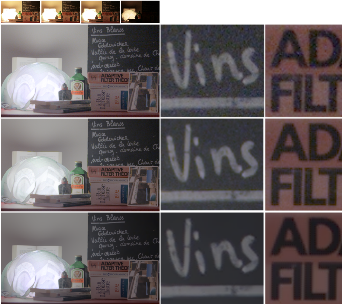
Figure 5.7: Real data. A static scene is acquired using a static camera. First row: Input images (JPEG version). Second row: Tone mapped reference image normalized by the exposure time. The saturated regions of the reference image were filled using the Poisson editing patch based approach described in Section 5.2.2. Third row: Tone mapped irradiance estimation by the MLE approach [Granados et al. 2010]. Fourth row: Tone mapped irradiance estimation of the proposed non local estimation approach. The result of the non local approach is less noisy than the one obtained using MLE. Thus releasing the alignment hypothesis does not have a significant impact on the algorithm performance. Recall that some demosaicking artifacts may appear due to the basic used technique. Please see electronic copy for better color and details reproduction.
