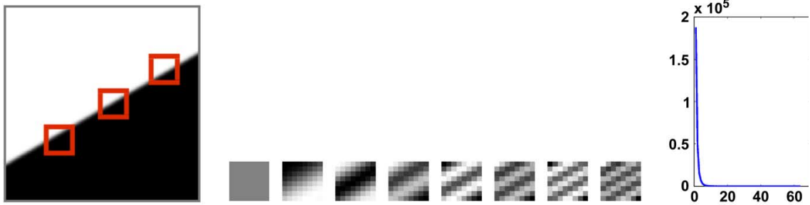
Figure 6.1: Left: Example of synthetic contour black-and-white image used to initialize the PLE method. Patches that touch the contour at different positions are randomly sampled from it and used to compute the corresponding class covariance matrix. Middle: First 8 eigenvectors of the covariance matrix corresponding to the largest eigenvalues. Right: Typical eigenvalues used for initialization. Image from [Yu et al. 2012].
