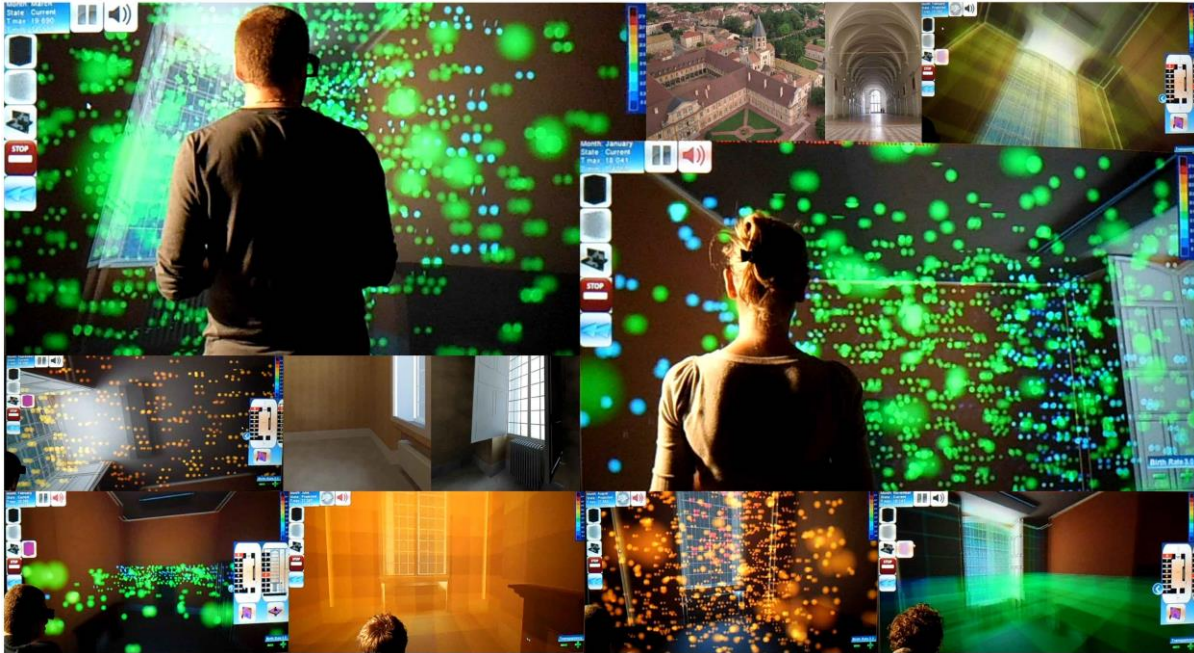
Figure 6.1. Images of TBS results of Gunzo room represented in VR. The application is intended to help building stakeholders to review their project design through thermal calculation results in order to obtain a sustainable building.
