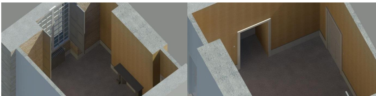
Figure 5.4. 3D view of Gunzo room in existing condition. Stone wall interior covered by wallpaper.
