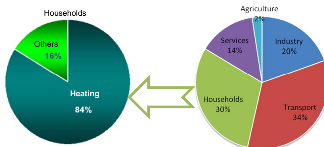
Figure 1.4. Most of household energy consumption in France is used for heating (Quenard, 2011).
