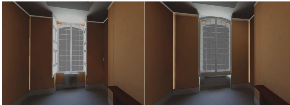
Figure 4.18. A 3D geometry enriched with texture mapping and exported to 3DViaStudio/Virtools. It shows 3D Model of Gunzo room before and after renovation.
