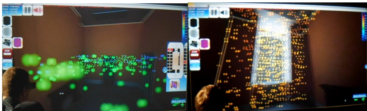
Figure 5.49. Visualization of layer particles. In normal cases, the simulation result will visualize the room completely filled with cubes or particles that indicate the temperature of the area they occupy. In order to make a better perception the both metaphors are also divided into 8 layers on each axis in the room. In this simulation, only two layers are shown at a time, a horizontal layer and a vertical layer.
