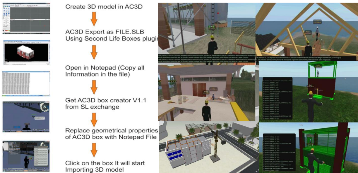
Figure 3.4. A building interactive modeling for construction education in VE proposed by Ku et al. (2011). The research using the AC3D software (3D modeling software) and Second Life platform (a game engine), to address the communication issues and effectively complement traditional teaching approaches and furthermore integrate with BIM to enhance construction education.
