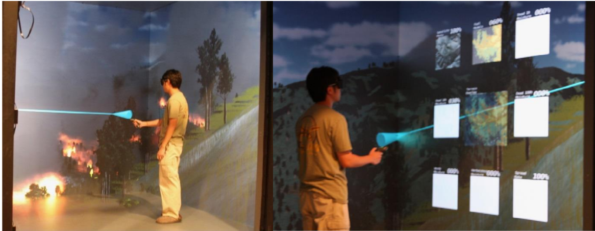
Figure 3.14. VFire running in a 6-sided CAVE-like environment. The data layers can be modified by the user using joystick.
