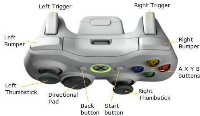
Figure 4.26. Xbox Controller Input.
