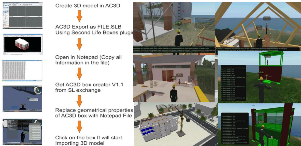
Figure 3.4. A building interactive modeling for construction education in VE proposed by Ku et al. (2011). The research using the AC3D software (3D modeling software) and Second Life platform (a game engine), to address the communication issues and effectively complement traditional teaching approaches and furthermore integrate with BIM to enhance construction education.
