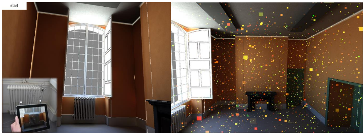
Figure 5.39. Gunzo room in existing condition and TBS results with visualization particles (Sept. 6 th 14:15)
