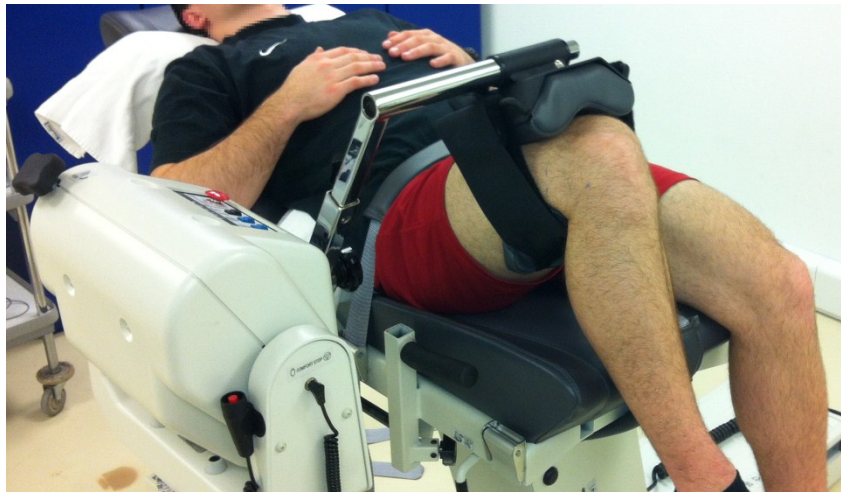
Figure 3. Test settings for hip flexor muscle strength evaluation on an isokinetic dynamometer.
