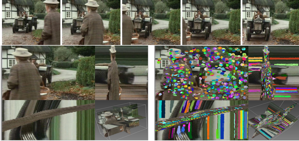
Figure 3.12: Top Row: Displays five images of a sequence from [Brox 2010]. Bottom Row: Left image displays the same video as a 3D volume as in Fig. 3.1, with an additional bottom right corner showing the 3D position of the xt and yt slices. Right image displays all fibers found, in different colors. Notice that the fibers are well stopped near occlusion vicinity, despite high similarity in color of the tractor and the lady.
