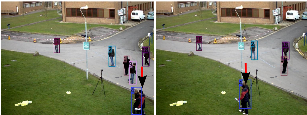
Figure 7.7: Missing persons in annotation : Frame numbers 509 and 526 from PETS S2L1 video. The person below the red arrow is not annotated for a length of 17 frames.
