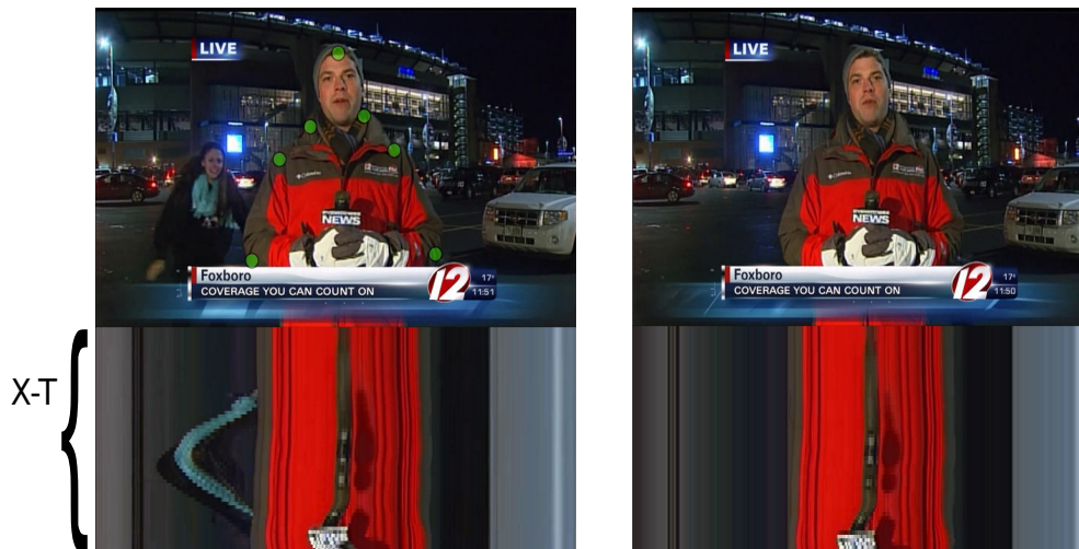
Figure 4.16: Inpainting task. Left: original video (top) and xt slice (bottom) showing trajectories. Right: Our result. Clusters of fibers were computed and selected with only 7 mouse clicks to distinguish the disturbing girl from the reporter and background. The girl was removed and the hole was filled by extending the background fibers in time.
