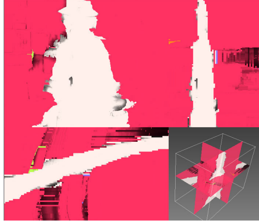
Figure 3.17: Displays extended fibers merged at a higher hierarchy. For a simple illustrative viewing, we fuse fibers which have similar motion. The next section 3.5 will elaborate on merging fibers. Darker regions refer to a low reliability of segmentation.
