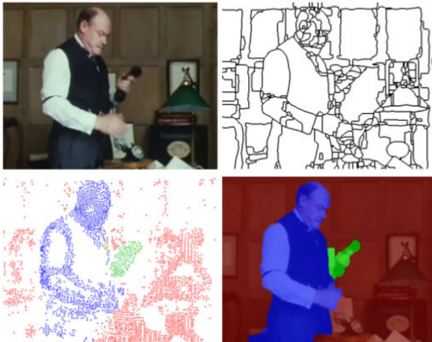
Figure 2.15: Output from [Ochs 2011]. This approach uses the sparse labeling information from [Brox 2010] ( Bottom Left ) and utilizes information from superpixels and gradients to obtain the final labeling ( Bottom Right ).
