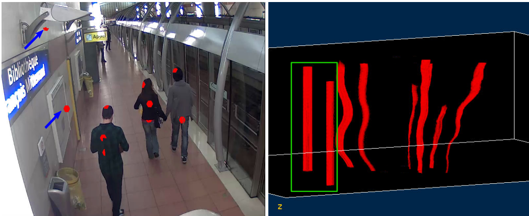
Figure 3.3: Sample fibers. Left: Red colored patches show sample fibers on one frame. Right: Sample fibers are displayed by a 3D visualizer (ImageJ). The Green box encloses two straight fibers which are formed by the patches on the background. Patches forming straight fibers are marked by the blue arrows on the left image.
