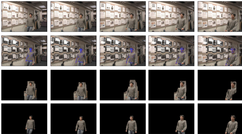
Figure 2.16: Background Subtraction in freely moving cameras from [Sheikh 2009]. First Row: Input image frames. Second Row: Clustered point tracks with blue representing foreground trajectories. Third Row: Estimated foreground labeling. Fourth Row: Groundtruth for foreground separation.
