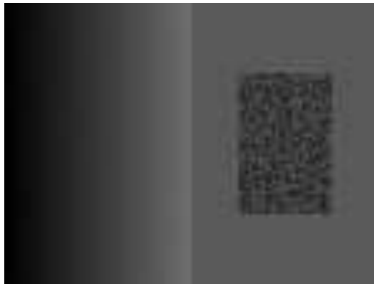
Figure 2.3: Image showing the importance of non local criterion which can segment above into three regions. There are three segments in an image with a rectangular-shaped intensity ramp in the left half, a constant intensity region with a hole of a high variability rectangular region.
