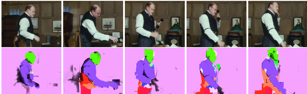
Figure 4.7: First Row: Sample input image frames (12, 24, 46, 53, 66) from marple13 sequence by [Brox 2010]. Bottom Row: After 5 steps of hierarchical merging. Parts of the foreground and background are undistinguishable during the first frames ( until the 12th frame , i.e. the leftmost image in the above figure ) of the video (same color). Yet, the two objects follow later significantly different trajectories, which enables us, when propagating this information back in time, to separate them as different fibers in all frames ( cf. section 3.3.2).
