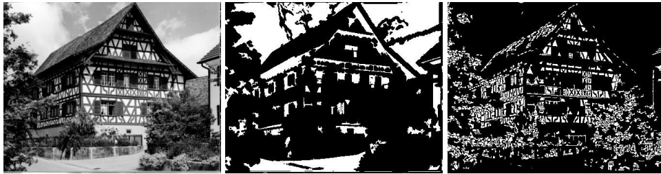
Figure 2.2: Different automatic seed selection sources. Left : Input Image. Center : Seeds obtained from homogeneity criteria. Right : Seeds obtained from edges in Input image (Seeds are shown as white regions).
