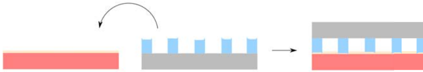
Figure 4.19: \mu -pillar / LSC coupling. \mu -pillar are softly put down on a LSC plate on which buffer resist has been spin-coated.
