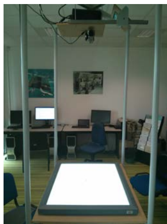
FIGURE B.1: SurMap prototype with depth sensor for 3D gesture recognition
