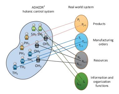
Figure 4.2 – Mapping ADACOR<sup>2</sup> Holons Into Real System
