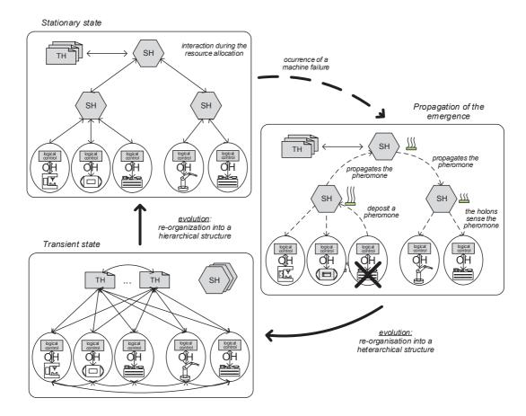
Figure 2.6 – Adaptation Mechanism in ADACOR Supporting a Hybrid Control Architecture
