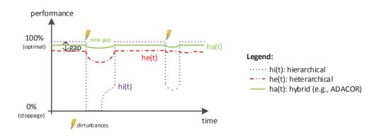
Figure 1.1 – Performance Behaviour of Different Classical Control Structures
