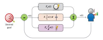
Figure 5.7 – Nervousness control mechanism based on PID controllers
