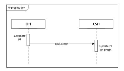
Figure B.1 – AUML PF Propagation
