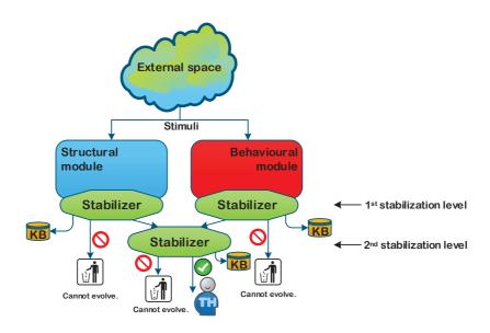
Figure 4.24 – Stabilization Mechanism Embedded in ADACOR<sup>2</sup> Holons
