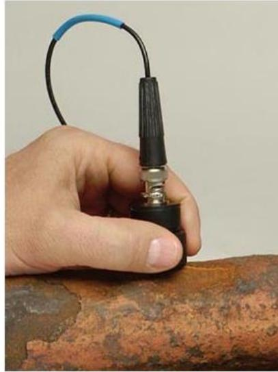
Figure I-15: Sonde Ultrasonique [45]
