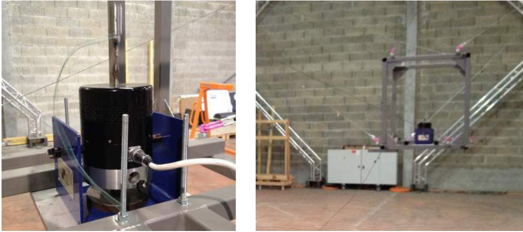
Fig. 4.6 Modal analysis of the CoGiRo by the shaker
