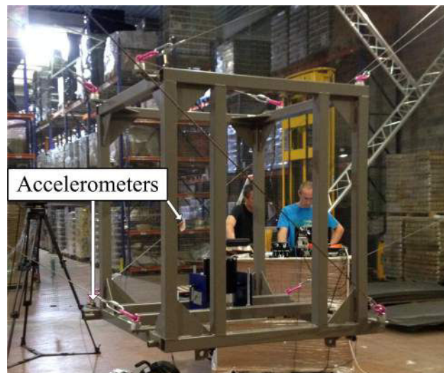
Fig. 4.11 Free vibration experiment at an emergency stop
