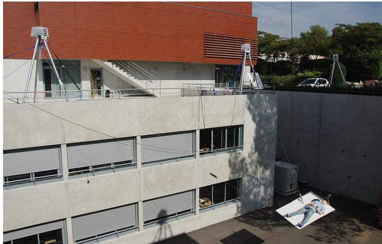
Fig. 1.6 The MARIONET-CRANE for emergency rescue by [Merlet 2010]
