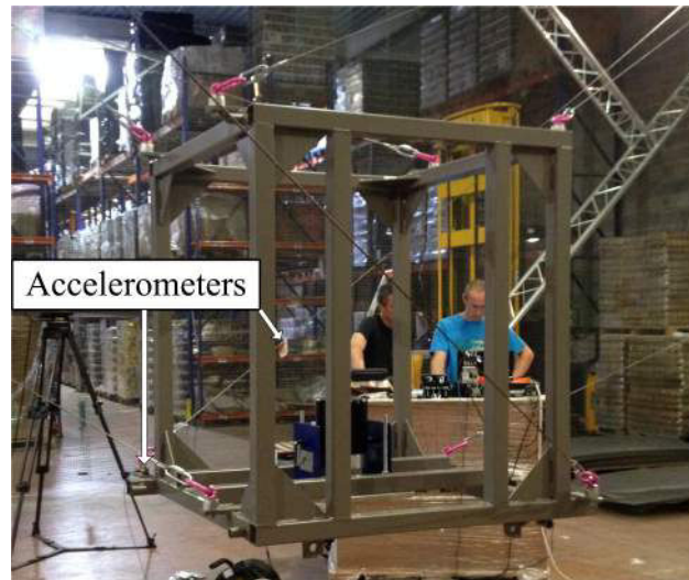
Fig. 4.11 Free vibration experiment at an emergency stop
