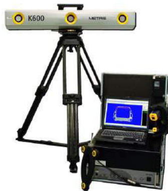
Fig. A.2 The Nikon K-600 camera system
