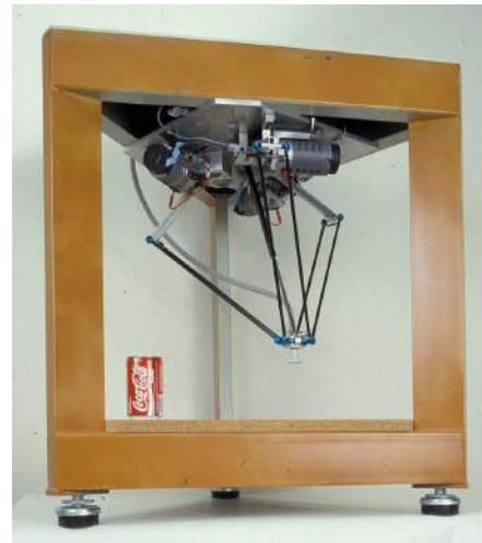
(b) The first Delta robot [Clavel 1991]
