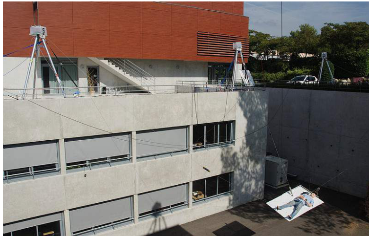
Fig. 1.6 The MARIONET-CRANE for emergency rescue by [Merlet 2010]
