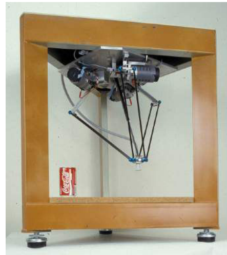
(b) The first Delta robot [Clavel 1991]
