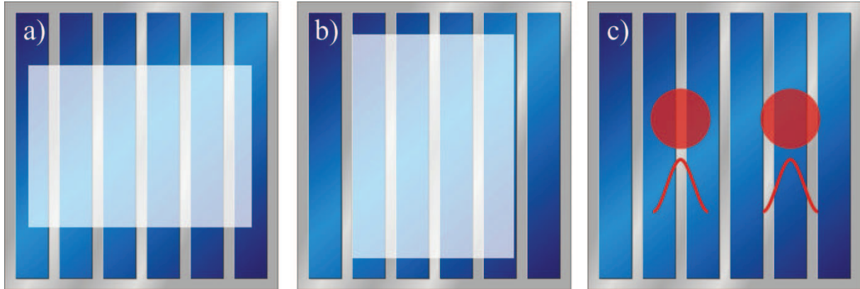
Figure III.27. Different spot sizes and their influence on the measured reflectivity. The same spot can produce different response, depending on the orientation (a and b) and also on the distribution of the intensity in the spot (c) which is particularly important for laser spots.
