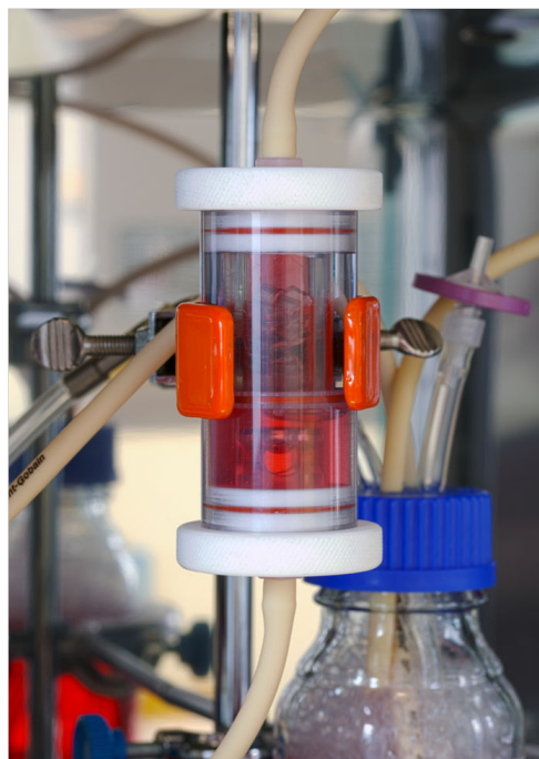
Figure 2.3 – The perfusion bioreactor. Left : Schematic representation of (A) indirect perfusion, (B) direct perfusion [Rauh et al., 2011]. Right : Photography of a perfusion bioreactor prototype used in our team.
