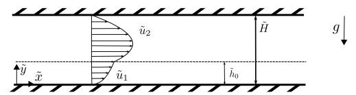
Figure 5.3: Uniform flow of a two-layer in an horizontal channel.
