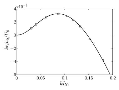
Figure 7.4: Linear growth rate of a gravity-driven film of water-glycerin down a  $6.4^{\circ}$  inclined plane. Dimensionless numbers: Re = 8.5, We = 0.048, Fr = 0.31. Solid line: solution of the long-wave dispersion relation (5.22); squares: computational analysis.
