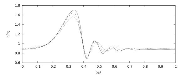
Figure 8.3: Film thickness at  $t=0.75\ s$  normalized to the flat equilibrium value versus stream-wise direction normalized with the wavelength. Convergence in the x-direction for three different meshes. Solid line: mesh 4 in Table 8.2; dashed line: mesh 2; dotted line: mesh 1. Physical parameters are detailed in the caption of Figure 8.2.
