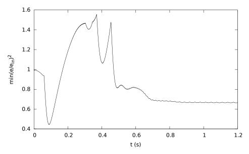
Figure 6.6: Time evolution of the minimum characteristic velocity  $e^2$  normalized with the initial value  $e_{in} = 2.5 \cdot 10^{-4} \ m^2 s^{-2}$ . Two-layer flow with dimensionless numbers:  $Re_1 = 4.48$ ,  $Re_2 = 36.8$ , Fr = 0.93, We = 0.002, and geometry given by  $\tilde{H} = 0.39 \ mm$  and  $\lambda = 26 \ mm$ . After 0.7 s periodic waves appear.
