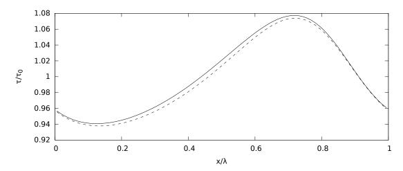
Figure 7.16: Interfacial shear stress normalized with the uniform value  $\tau_0 = 0.61 \ Pa$ , corresponding to film thickness of Figure 7.15. Solid line: asymptotic expansion; dashed line: code SWANS. Physical and numerical parameters in the caption of Figure 7.15.
