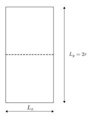
Figure 7.10: Geometry of the plane Poiseuille flow. Channel length is  $L_x = 1 \ mm$  and the height is  $L_y = 2r = 2 \ mm$ .
