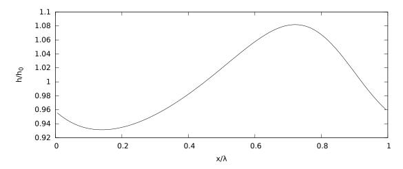
Figure 7.15: Film thickness at t=0.03~s from SWANS. Dimensionless numbers:  $Re_1=8.7, Re_2=71.3.$ Pressure drop:  $\Delta p=62~Pa$ . Mesh size:  $\Delta_x=81.2~\mu m, \Delta_y=10.8~\mu m$ .
