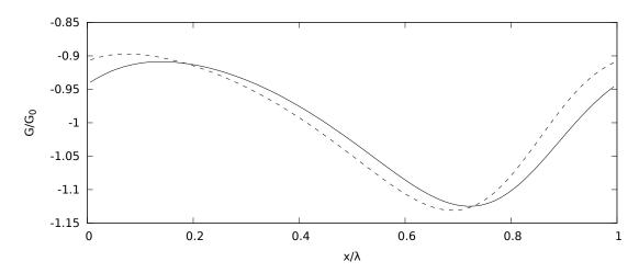
Figure 7.17: Space evolution of the interfacial pressure gradient normalized with the uniform value  $G_0 = 4769 \ Pa \ m^{-1}$ , corresponding to film thickness of Figure 7.15. Solid line: asymptotic expansion; dashed line: code SWANS. Physical and numerical parameters in the caption of Figure 7.15.
