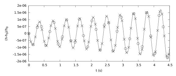
Figure 7.1: Temporal evolution of the dimensionless film thickness at imposed wavelength  $\lambda = 70 \ mm$ , and convergence of three mesh sizes: 40 (circles), 80 (cross) and 160 (solid line) cells in the domain. Dimensionless numbers: Re = 8.5, We = 0.048, Fr = 0.31.
