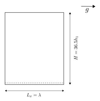
Figure 8.12: Geometry sketch (with a 10 : 1 scaling) of the vertical test, where  $L_x = 5.2 \ mm$  and  $H = 6.37 \ mm$ . Dotted line expresses the equilibrium film thickness.
