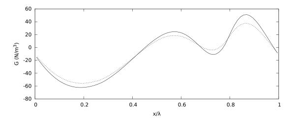
Figure 8.22: Interfacial pressure gradient space evolution. Comparison between SWANS (dotted line) by adding the dissipative term  $2\partial_{xx}q$  and without (solid line). Physical parameters are detailed in the caption of Figure 8.13.
