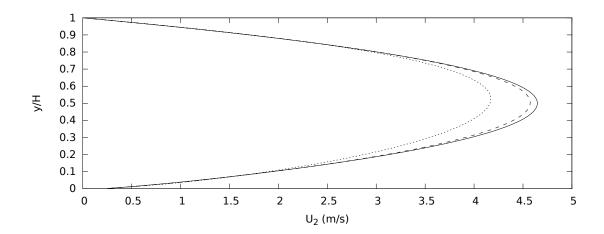
Figure 8.15: Gas velocity profiles at  $t=0.25\ s$ . Convergence of three different meshes. Solid line: mesh 7 in Table 8.3; dashed line: mesh 6; dotted line: mesh 5. Physical parameters are detailed in the caption of Figure 8.13.
