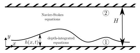
Figure 6.1: Sketch of the performed computational investigation. Indices 1 and 2 refer to liquid and gas phases, respectively.
