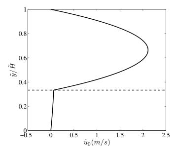
Figure 5.4: Uniform velocity profile of an air-water flow in a channel:  $\tilde{Q} = 4.06 \cdot 10^{-4} \ m^2 s^{-1}$ ,  $\tilde{L} = 26 \ mm$ ,  $\tilde{H} = 0.39 \ mm$ , r = 0.001 and m = 0.01. Dashed line is the flat interface.
