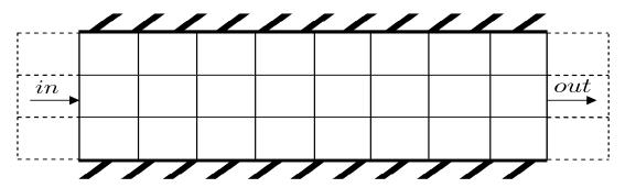
Figure 6.7: Sketch of the gas mesh and definitions of periodic boundary conditions.
