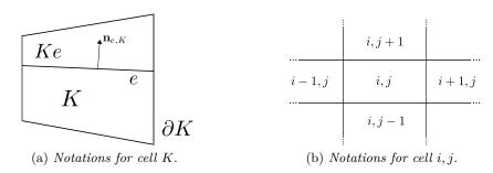
Figure 6.8: Two different cell notations for the low-Mach scheme used in this work.
