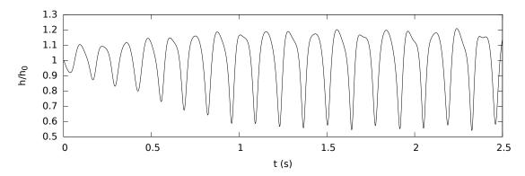
Figure 7.8: Temporal wave dynamics and saturated waves, spatially periodic, of a falling water-glycerin film down a  $6.4^{\circ}$  inclined plane. Data correspond to Liu & Gollub experiments:  $Re=19.3, We=35, f=7~Hz~(\lambda=3~cm$  in the performed computational analysis).
