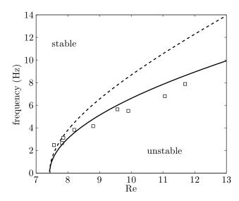
Figure 5.6: Neutral stability curve for gravity-driven water-glycerin films down a 6.4° inclined plane. Solid line: Orr-Sommerfeld theory; dashed line: first-order long-wave model of Chapter 3, subject to gravity only; squares: experiments of Liu, Paul and Gollub [48, 47].
