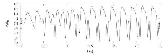
Figure 7.5: Temporal wave dynamics and saturated waves, spatially periodic, of a falling water-glycerin film down a  $6.4^{\circ}$  inclined plane. Data correspond to Liu & Gollub experiments:  $Re=19.3, We=35, f=4.5 \ Hz \ (\lambda=5 \ cm$  in the performed computational analysis).
