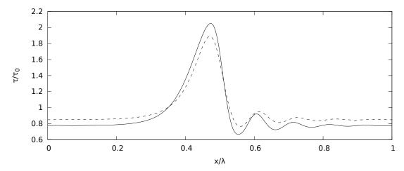
Figure 8.7: Space evolution of interfacial shear stress normalized to the uniform condition. Comparison between the two-layer long-wave model of Dietze & Ruyer-Quil (dashed line), Figure 8(c) of [25] after appropriate scaling, and SWANS (solid line). Physical parameters are detailed in the caption of Figure 8.2. Data of the two-layer long-wave model courtesy of G. Dietze.
