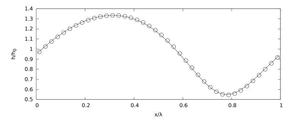
Figure 8.14: Film thickness versus normalized wavelength at  $t=0.235\ s$ . Convergence of two different meshes. Solid line: mesh 6 in Table 8.3, circles: mesh 5 in Table 8.3. Physical parameters are detailed in the caption of Figure 8.13.
