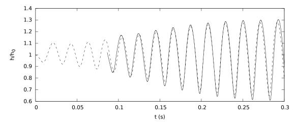
Figure 8.19: Film thickness time evolution. Comparison between SWANS (solid line) by adding the dissipative term  $2\partial_{xx}q$ , and DNS provided by G. Blanchard by means of Slosh (dashed line). Physical parameters are detailed in the caption of Figure 8.13.
