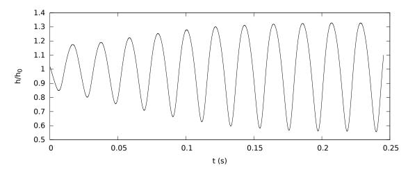
Figure 8.13: Time evolution of normalized film thickness for the vertical flow. Dimensionless numbers:  $Re_1=16.5$  and  $Re_2=1972$ , Fr=5.65, We=0.021. Uniform flow:  $\tau_{i0}=0.03$  Pa,  $u_0|_h=0.15$  m  $s^{-1}$ .
