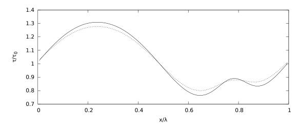
Figure 8.21: Interfacial shear stress space evolution. Comparison between SWANS (dotted line) by adding the dissipative term  $2\partial_{xx}q$  and without (solid line). Physical parameters are detailed in the caption of Figure 8.13.
