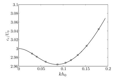
Figure 7.3: Wave celerity of a gravity-driven film of water-glycerin down a  $6.4^{\circ}$  inclined plane. Dimensionless numbers: Re = 8.5, We = 0.048, Fr = 0.31. Solid line: solution of the long-wave dispersion relation (5.22); squares: code SWANS.
