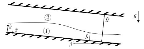
Figure 2.5: Definition of the geometry of a liquid film (index k=1) sheared by a gas flow (index k=2) in an inclined channel.
