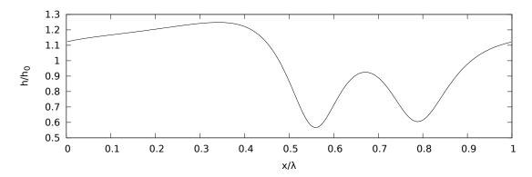
Figure 7.6: Shape of saturated waves of a falling water-glycerin film down a 6.4° inclined plane, at t=1.6~s. Data correspond to Liu & Gollub experiments: Re=19.3, We=35, f=4.5~Hz ( $\lambda=5~cm$  in the performed computational analysis).
