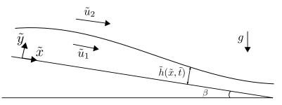
Figure 2.4: Sketch of a liquid film sheared by a gas flow and definition of the coordinate system. For falling films,  $\tilde{u}_2 = 0$ .
