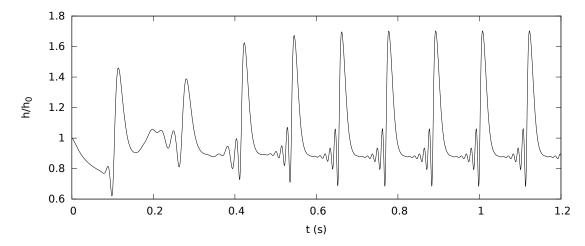
Figure 8.2: Time evolution of the film thickness normalized with the uniform flow. Dimensionless numbers:  $Re_1 = 4.48, Re_2 = 36.8, Fr = 0.93, We = 2 \cdot 10^{-3}$ . Uniform pressure gradient and shear stress:  $G_0 = -\Delta p/L = 2461.5 \ Pa \ m^{-1}, \tau_{i0} = 0.32 \ Pa$ .
