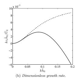
Figure 5.5: Dispersion curves from (5.22) for a water-glycerin gravity-driven film down an inclined plane of  $\beta=6.4^{\circ}$ . Dimensionless numbers: Re=8.5, Fr=0.316, We=0.048. Case with surface tension (solid line) and without surface tension (dashed line).
