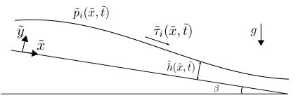
Figure 3.2: Sketch of a liquid film subject to interfacial shear stress and pressure, and the gravity.
