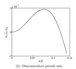
Figure 5.9: Dispersion curves from (5.36) for an air-water system flowing in a confined channel neglecting the gravity:  $\tilde{H} = 0.39 \ mm$ ,  $\tilde{h}_0 = 0.13 \ mm$ ,  $\tilde{u}|_h = 0.06 \ m\ s^{-1}$ . Dimensionless numbers:  $Re_1 = 4.48$ ,  $Re_2 = 36.8$ , Fr = 0.93, We = 0.002.
