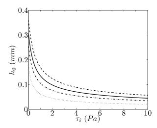
Figure 5.7: Equilibrium thickness versus shear stress from (5.26), for a water film down a  $\beta=4^{\circ}$  inclined plane, and for several Reynolds numbers: Re=2 dotted line, Re=6 dash-dot line, Re=10 solid line, Re=16 dashed line.
