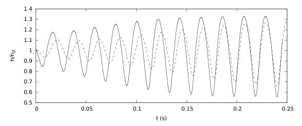
Figure 8.16: Film thickness time evolution. Comparison between SWANS (solid line) and DNS provided by G. Blanchard by means of Slosh (dashed line). Physical parameters are detailed in the caption of Figure 8.13.
