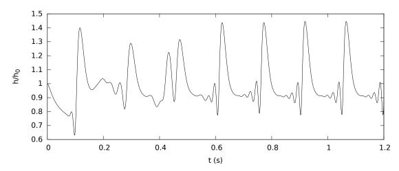
Figure 8.10: Time evolution of the film thickness normalized with the equilibrium film state obtained by means of the two-layer depth-integrated equations of Chapter 4. Physical parameters are detailed in the caption of Figure 8.2.
