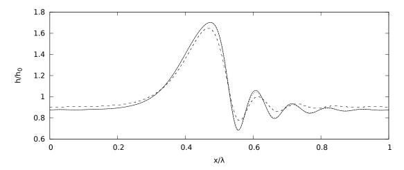
Figure 8.23: Film thickness time evolution of the horizontal two-layer flow. Comparison between SWANS (dotted line) by adding the dissipative term  $2\partial_{xx}q$  and DNS provided by Dietze & Ruyer-Quil with OpenFOAM (dashed line). Solid line is solution by SWANS without second-order dissipative contribution. Physical parameters are detailed in the caption of Figure 8.2.
