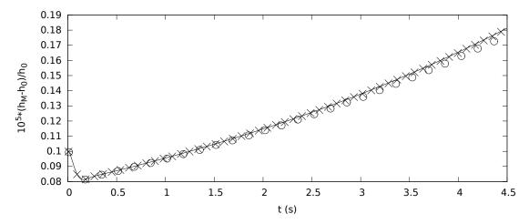
Figure 7.2: Temporal evolution of the dimensionless maximum film thickness  $h_M$  in the domain at imposed wavelength  $\lambda=70~mm$ , and convergence of three mesh sizes: 40 (circles), 80 (cross) and 160 (solid line) cells in the domain. Dimensionless numbers: Re=8.5, We=0.048, Fr=0.31.
