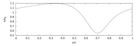
Figure 7.9: Shape of saturated waves of falling water-glycerin film down a  $6.4^{\circ}$  inclined plane, at t=1.6~s. Data correspond to Liu & Gollub experiments:  $Re=19.3, We=35, f=7~Hz~(\lambda=3~cm$  in the performed computational analysis).
