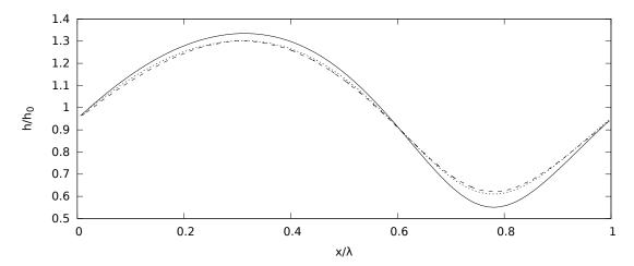
Figure 8.20: Film thickness space evolution of the traveling wave. Comparison between SWANS (dotted line) by adding the dissipative term  $2\partial_{xx}q$ , and DNS provided by G. Blanchard by means of Slosh (dashed line). Solid line is solution by SWANS without second-order dissipative contribution. Physical parameters are detailed in the caption of Figure 8.13.
