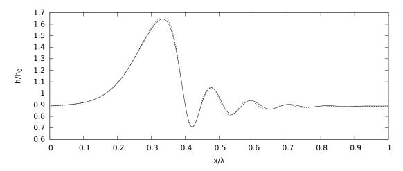
Figure 8.4: Film thickness at  $t=0.75\ s$  normalized to the flat value versus stream-wise direction normalized with the wavelength. Convergence in the y-direction for two different meshes. Solid line: mesh 3 in Table 8.2; dotted line: mesh 2. Physical parameters are detailed in the caption of Figure 8.2.
