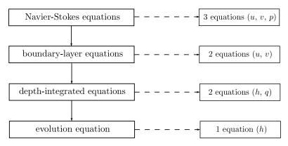
Figure 2.3: Levels of modeling approximation for falling liquid films.
