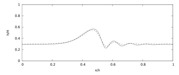
Figure 8.5: Traveling wave in the channel, and comparison between DNS of Dietze & Ruyer-Quil (dashed line), Figure 7(a) of [25], and SWANS (solid line). Physical parameters are detailed in the caption of Figure 8.2. DNS data courtesy of G. Dietze.
