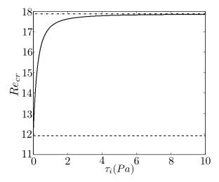
Figure 5.8: Critical Reynolds number versus shear stress from (5.30) and (5.31), for a water film down a  $\beta = 6^{\circ}$  inclined plane. Dashed line is the limit of gravity-driven films, i.e.  $\tau_i = 0$ ; dash-dotted line is the limit of an infinite  $\tau_i$ .
