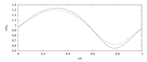
Figure 8.18: Film thickness space evolution of saturated non-linear waves. Comparison between SWANS (solid line) and DNS provided by G. Blanchard by means of Slosh (dashed line). Physical parameters are detailed in the caption of Figure 8.13.
