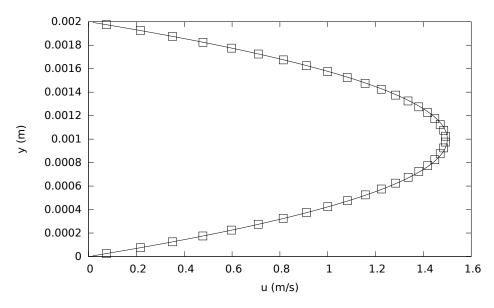
Figure 7.11: Poiseuille velocity profile at t = 0.4 s on a fixed grid and comparison with the exact solution. Squares: mesh 10x40; solid line: exact profile.
