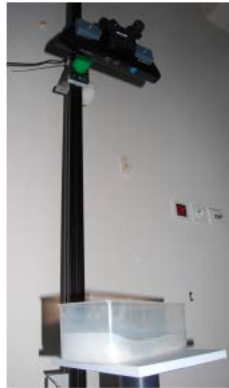
Figure 7.1 – Experimental set with the Kinect sensor.
