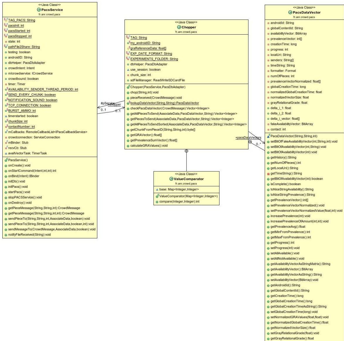
Figure B.2: PePiT communication module UML class diagram.
