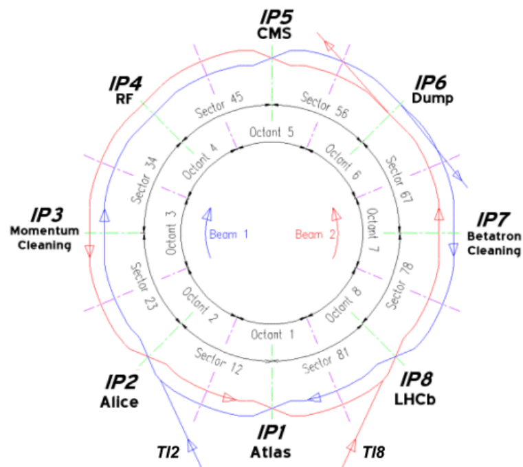
Figure 2.14: Schematic of the LHC layout with marked insertion regions, sectors and octants. Figure from [CER13].
