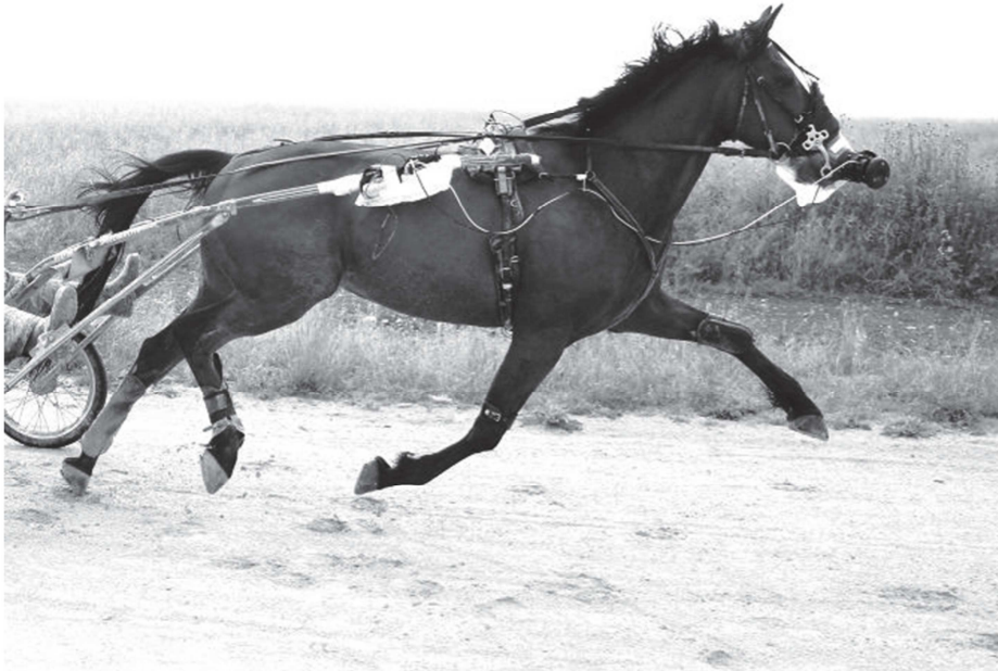
Supplementary Figure S1 A Standardbred trotter exercising a parcours with the Equimask connected to the portable gas analyser K4b 2 with his battery fixed on the sulky.
