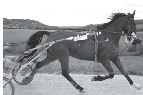
Fig. 1 A Standardbred trotter exercising a field test with the Equimask connected to the portable gas analyser K4b 2 with his battery fixed on the sulky.
