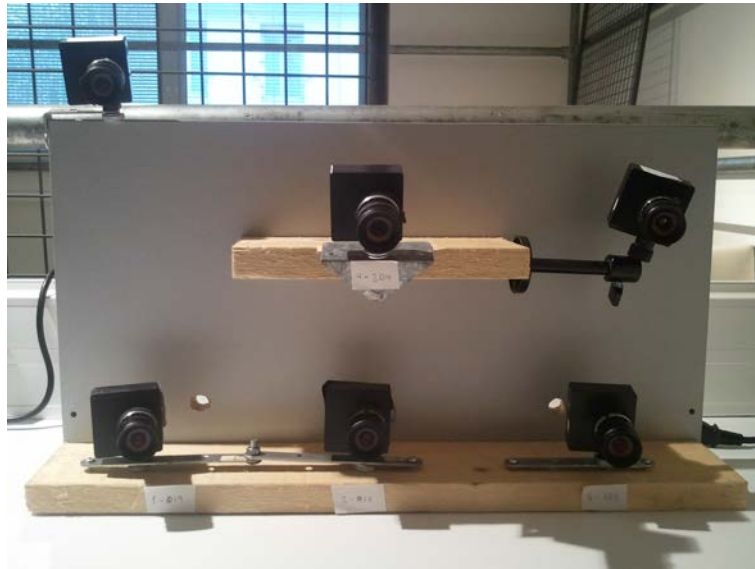
Figure 2.7: Experimental setup composed of 6 DVS cameras.
