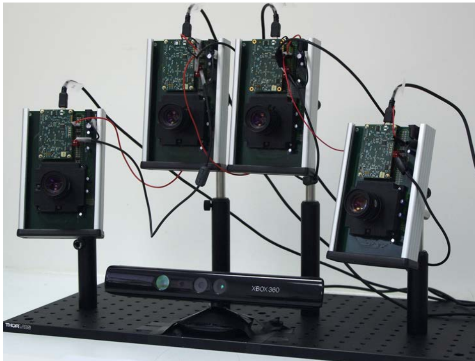
Figure 4.9: Multicamera setup composed of three ATIS sensors and a Microsoft Kinect sensor for ground-truth.
