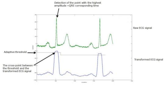
FIG. 3.3 - Example of QRS detection.
