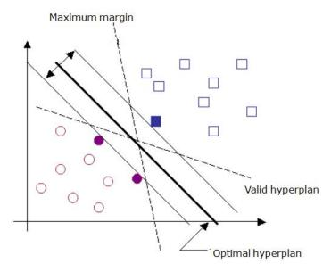
FIG. 3.12 - Classification for optimal hyperplane.
