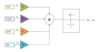
$\pmb{\text{FIG. 6.9 -} \text{Optimal fusion rule applied to time series extracted from pressure signal.}}\\$
