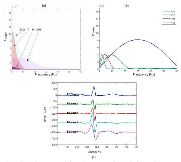
**FIG. 3.6 -** (a) Spectral representation of a beat and its components: the P, QRS and T wave. (b): presentation of different filters (W21 to W24) applied to the signal to identify a specific frequency range. (c): results from the application of these filters on an initial beat: obtaining a beat decomposed into four specific levels (1-4).
