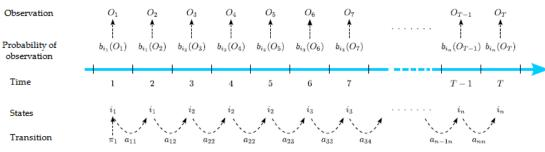
FiG. C.3 – Principle of hidden Markov Model (Altuve, 2011).
