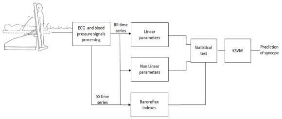
FIG. 4.1 - Block diagram of the proposed approach for syncope prediction.
