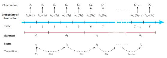
FiG. C.4 – Principle of hidden semi-Markov Model (Altuve, 2011).
