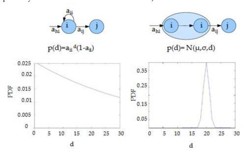
**FIG.6.10-** Difference between HMM / HSMM on the modeling of the time spent in a state: in the left panel a state in HMM whose PDF of duration follows a geometrical distribution function, in the right panel a state of HSMM of which the PDF of duration follows a normal distribution with  $\mu$  and  $\sigma$  parameters.
