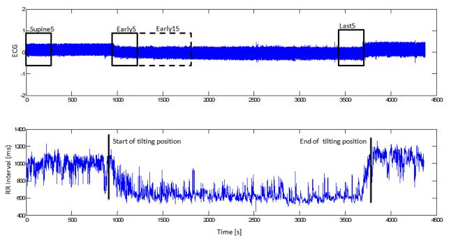
**FIG. 4.4** - Example of an ECG recording with the different time intervals used for analysis, for a subject with negative response (a) and the corresponding RR time series (b). The RR-interval time series corresponding to each window are used to extract the features that will be used for classification.
