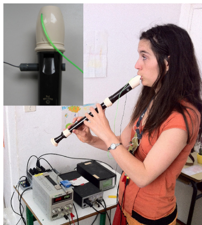
FIGURE 7.5: Experimental setup with the adapted alto Zen-On recorder, allowing the measurement of both the pressure in the mouth of the recorder player and the acoustic pressure under the labium.
