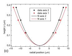
Figure 5.6: Determination of ROC using an interferometric measurement. (a): Interferometric microscope image of a microfabricated fibre facet ( $\emptyset 125\mu$ m). The white circle limits the region for the subsequent reconstruction. (b): Intensity cut of the image along axis 1. (c): Reconstructed profile cuts along the two axes. Parabola fits give  $R_1 = 250\,\mu$ m and  $R_2 = 210\,\mu$ m.
