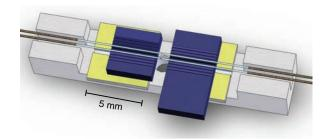
Figure 2.2: FFP cavity assembly (schematic). A support bridge made from ceramic (light grey) carries two shear piezos (yellow). Each piezo carries two silicon substrates (blue) into which the microfabricated fibres are glued.
