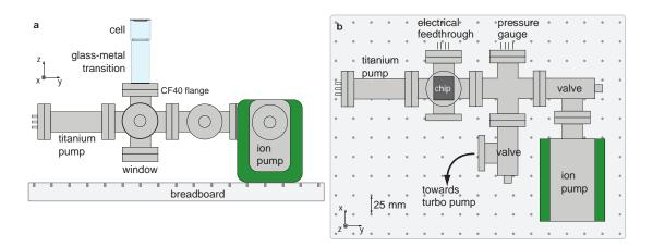
Figure 2.5: Vacuum setup. a) Side view. b) Top view. Adapted from [63].
