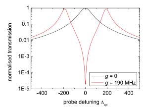
Figure 1.6: Transmission of the uncoupled (black) and coupled (red) atom-cavity system as a function of probe detuning with the cavity resonant to the atomic resonance  $(\Delta_{cp} = \Delta_{ap})$ . Our experimental parameters are  $(\gamma, \kappa, g) = 2\pi(3, 53, 190)$  MHz.
