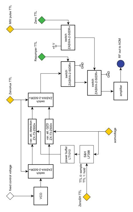
Figure C.1: Full schematic of the RF electronics to regulate the probe intensity during the QZD. Thick outlines indicate components from Minicircuits, thin outlines are electronic ICs. Yellow (green) diamonds indicate input from the real-time micro-controller (experiment control software).
