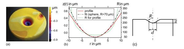
Figure 5.2: Analysis of microfabricated concave structures on an optical fibre. (a): 3d plot of the surface profile measured with an optical profilemeter. (c): Cut through the centre of the profile shown in (a). (c): Parameters used to characterise the profile. Our discussion concentrates on the radius of curvature (ROC) R. Adapted from [129].
