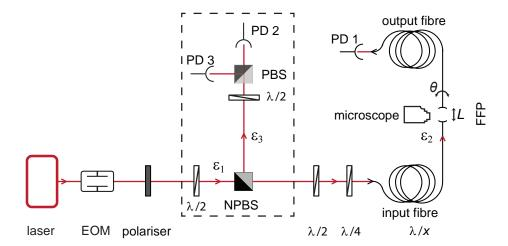
Figure 5.7: Schematic of the experimental setup to characterise mode splitting. The part within the dashed line is used to verify the polarisation angle  $\varepsilon_2$  of the light incident on the cavity as described in Appendix E.
