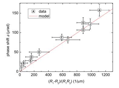
Figure 5.10: Differential phase shift  $\phi$  as a function of mirror geometry. The red line is the prediction of Equation 5.10.
