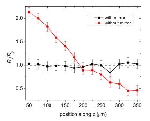
Figure 5.3: Ratio of horizontal to vertical radius of curvature  $R_x/R_y$  of CO<sub>2</sub> laser-machined structures (waist size about 32  $\mu$ m). The dichroic mirror used for alignment produces astigmatism so that the symmetry of the structures varies with the position on the beam axis z.
