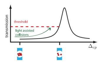
Figure 2.17: Principle of the atom number preparation scheme. The detuning between cavity and probe laser  $\Delta_{cp}$  changes proportionally to the number of off-resonant atoms in the cavity. Removing atoms until the transmission crosses a certain threshold allows us to prepare a well-defined atom number. Source: [45].
