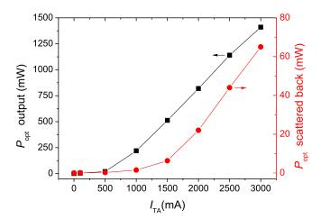
Figure 2.11: Optical power  $P_{\rm opt}$  at output (black squares) and scattered back into input direction (red circles) of the TA as a function of the operating current  $I_{\rm TA}$ . The TA was injected with 17 mW of optical power.
