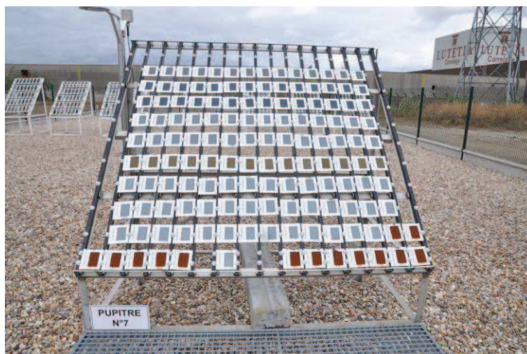
Fig. A.3. Sample desk in natural exposure site in Maizières, France. [Courtesy of ArcelorMittal R&D]
