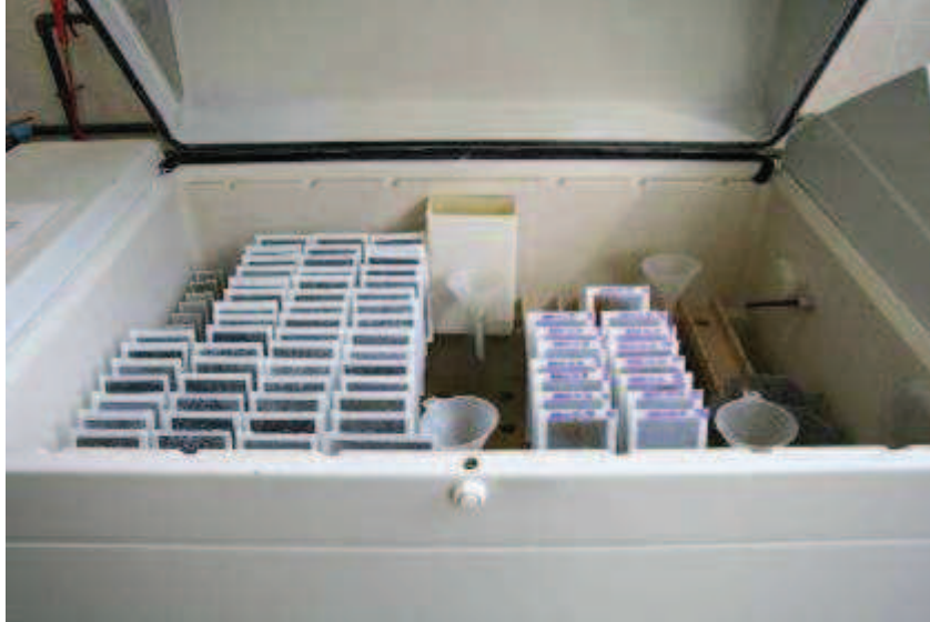
Fig. A.1. Climatic chamber used for accelerated corrosion tests. [Courtesy of ArcelorMittal R&D]
