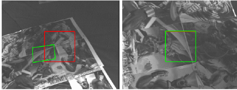
Figure 1.6 – Homography based visual servoing [Benhimane 06]. On the left is the initial image and right is the final image. The regions of interest in reference pose (red) and initial pose (green) are shown. On the right is the final image after the visual servoing where the current and desired regions of interest coincide
