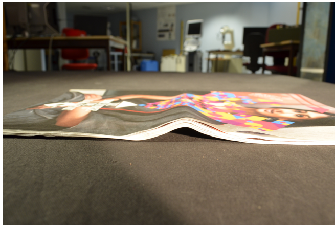
Figure 3.16 – Photograph of side-view showing non-planarity on one side of the target
