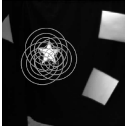
Figure 1.11 – Kernel placement in the acquired camera image (reproduced from [KalleM 09])
