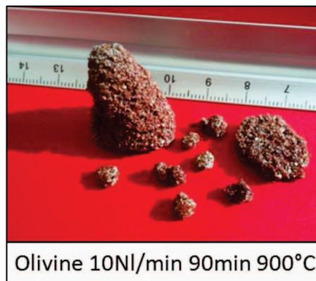
Figure V-11: Agglomerates after the fluidisation tests using olivine as bed material (process parameters; 1g of ash, air flow 10NL/min, time 90 minutes, T=900 °C)
