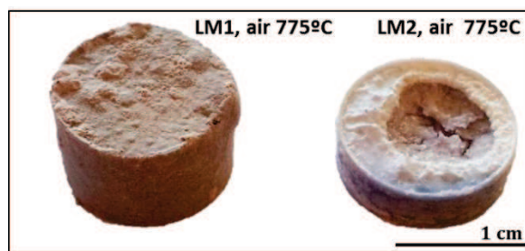
Figure II-37: LM1 and LM2 ashes heat treated in air at 775 °C for 6 hours
