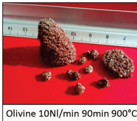
Figure V-11: Agglomerates after the fluidisation tests using olivine as bed material (process parameters; 1g of ash, air flow 10NL/min, time 90 minutes, T=900 °C)
