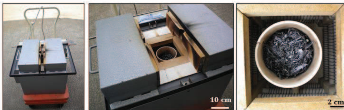
Figure II-20: Preparing miscanthus ashes at 400 °C in an open muffle furnace (Parmilleux, type: FP 1200)
