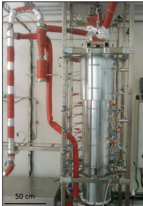
Figure V-21: Fluidized bed gasifier pilot at the laboratory LRGP, Nancy
