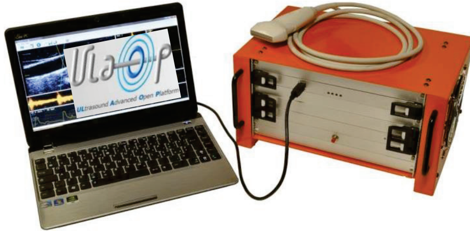
Figure 4.1: the Ula-Op scanner system used in the experimental measurements
