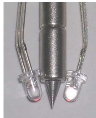
Figure 64: Adapted from [143]. On the left, photography of the FRMT experimental setup; illumination is achieved by the use of an optical fiber (top left on the photo). On the right, photography of the magnetic tip coupled with two LED to achieve better homogeneous illumination.
