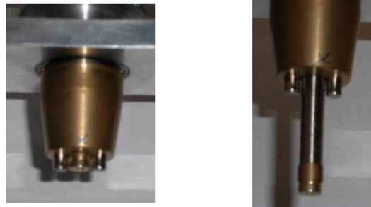
Figure 67: Photography of the magnet configuration in the hybrid magnetic tweezers setup. The smaller magnets are lowered on the left and are raised on the right. The height difference is of 25mm. The smaller magnets are separated from the main one by gaps of 0.2mm.
