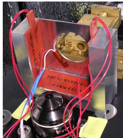
Figure 71: Photograph of the inside of the specimen holder in the hybrid magnetic tweezers setup. Three heating resistors are placed on the vertical sides of the inside of the holder. The temperature is measured by a platinum resistance thermometer placed directly under the holder, where the microfluidic chamber is positioned.
